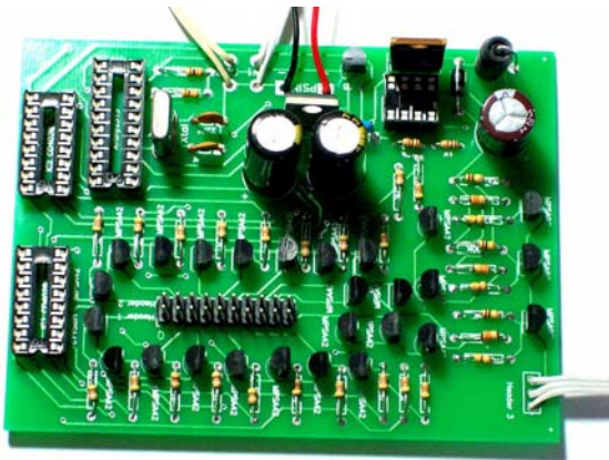
Figure 8 - Tall objects and wires soldered in
